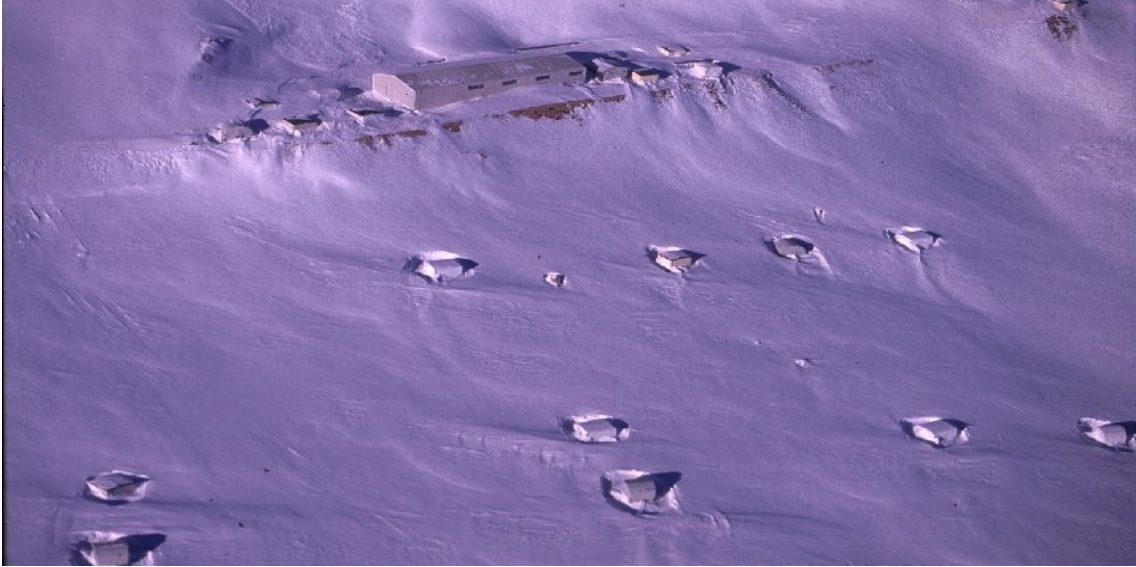
Figure 1: Aerial view of part of the EAS-TOP array during winter time. The e.m. modules are visible out of the snow; the muon detector is located inside the shed on top of the picture.
