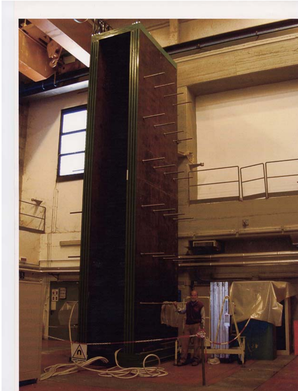
Figure 4: Full scale prototype of part of the dipole magnet constructed and tested at Frascati, as seen during construction.
