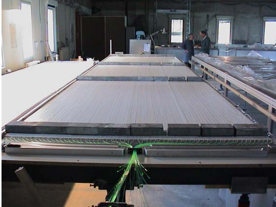
Figure 3: Full scale prototype of a module of the target tracker with plastic scintillators constructed and tested at Strasbourg.
