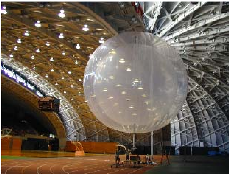
Figure 5: The nylon vessels, mounted for a pressure test
