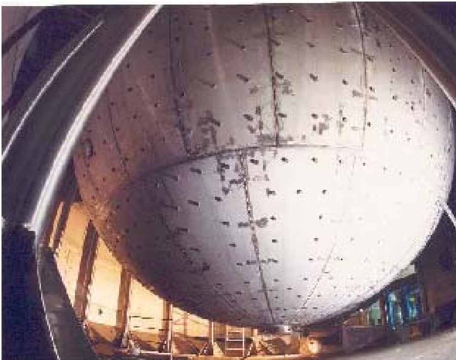
Figure 3: The stainless steel sphere as seen from the water tank
