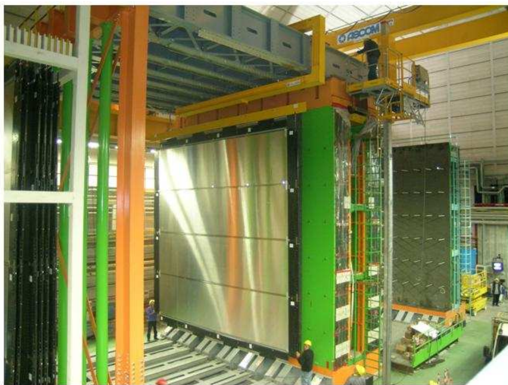
Figure 3: Insertion of the first Target Tracker wall inside the OPERA detector.
