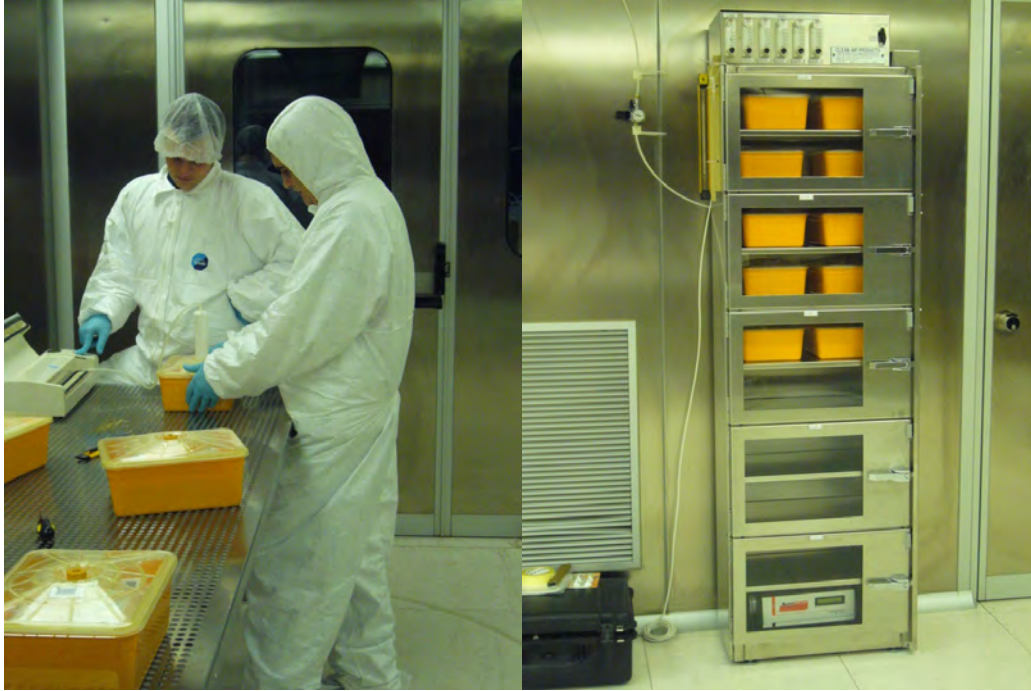
Figure 14: Storage of \text{TeO}_2 crystals at LNGS. Left: crystals as arrived (in their triple polyethylene bags) are stored inside vacuum boxes. Right: vacuum boxes containing crystals are stored in \text{N}_2 fluxed cupboard in the Permanent Storage Area (PSA)
