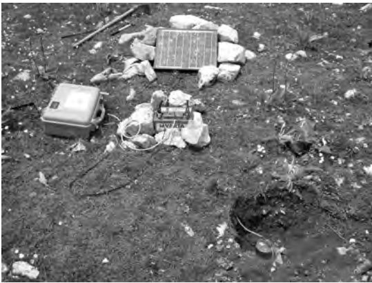
Figure 2: Left: FON6 station, as all the other FonArray ones, consisted in a Lennartz 3D-lite sensor, a solar panels and batteries power supply and a Lennartz MarsLite station with a GPS timing system. Right: FonArray geometric configuration. Stations GS02 and FON5 are also shown in the picture: after a short period of acquisition, they were dismantled.
