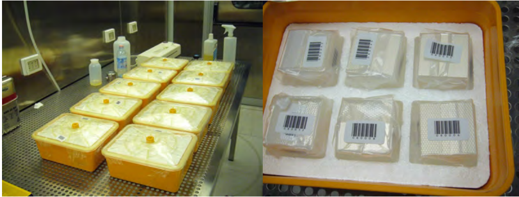
Figure 13: Delivery to LNGS of \text{TeO}_2 crystals transported by sea. Left: polyethylene vacuum boxes containing 59 crystals. Right: crystals in their triple polyethylene vacuum bags
