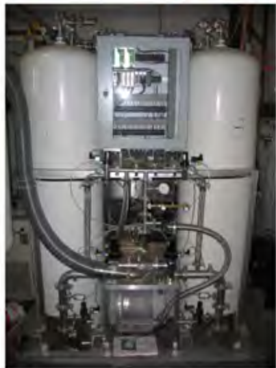
Figure 7: Top: the activation oven (LNGS - Hall di Montaggio, WarP Area). Middle: a (small) test cartridge (Trigon+Zeolite content) inside the oven for activation process. Bottom: Picture of the first stage VSA (Vacuum Swing Adsorption) purification unit as installed at the Reliant Dry Ice Plant in Buxton, New Mexico. Top center: the control system of the two-stage VSA purification system.
