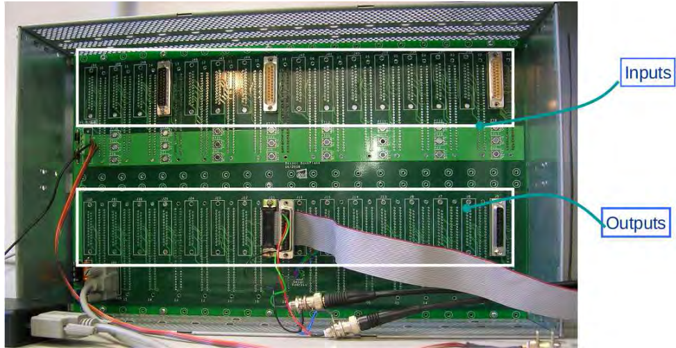
Figure 16: Back-plane for the Thomson antialisaing filter.
