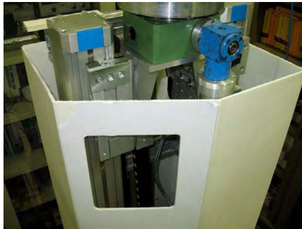
Figure 10: The paper prototype of the garage (now ordered) containing the tower elevator with its servo system for rotation and z-movement (the remote control cabin is not shown).
