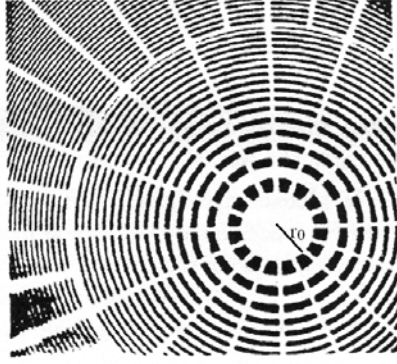
Figure 7: TEM image (x100) of a part of the gold zone plate. 1010 \mu\text{m} diameter and 22.5 \mu\text{m} r_0 .
