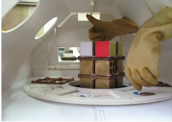
Figure 11: Ergonomic studies with mech-box paper mock-up.
