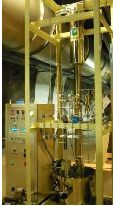
Figure 2: Picture of the Kr distillation column in commissioning.
