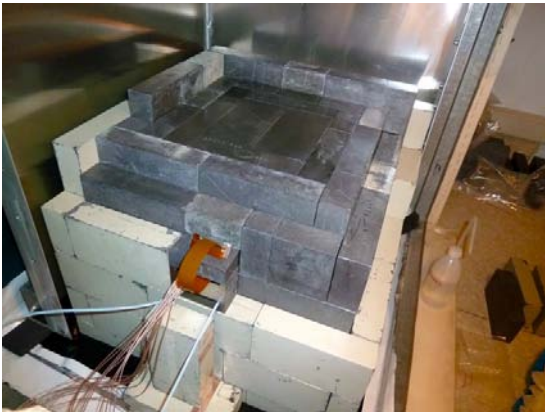
Figure 4: Nearly finished lead castle with HV-, capton-signal cable and N 2 pipes
