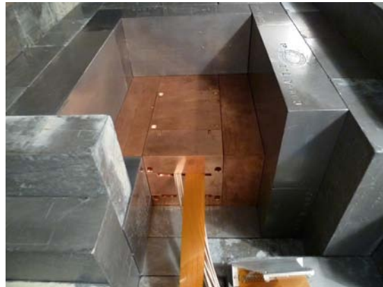
Figure 5: Cu-Nest surrounded with ULA lead and installed detector layer
