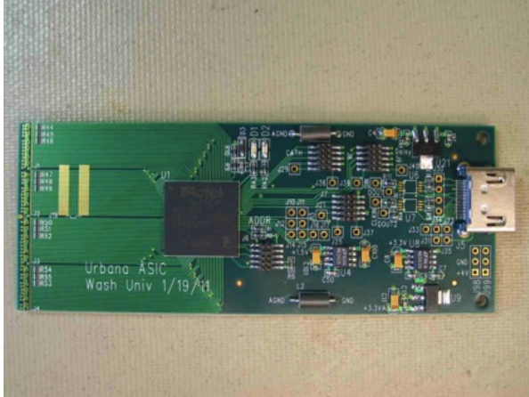
Figure 15: Custom data acquisition board developed by WUSTL for readout of the 350\ \mu\text{m} and 700\ \mu\text{m} detectors supported by the 2048-channel UIUC/Ajat ASIC.
