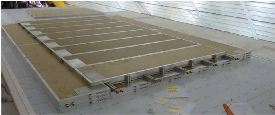
Figure 6: The GERDA plastic veto mounted on top of the clean room. 36 panels are installed and secured with steel wires and a metal fence.
