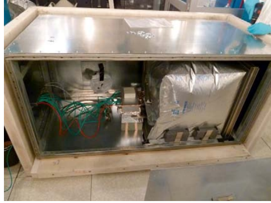
Figure 3: Opened setup with radon tight foil, EMI shield and neutron shield
