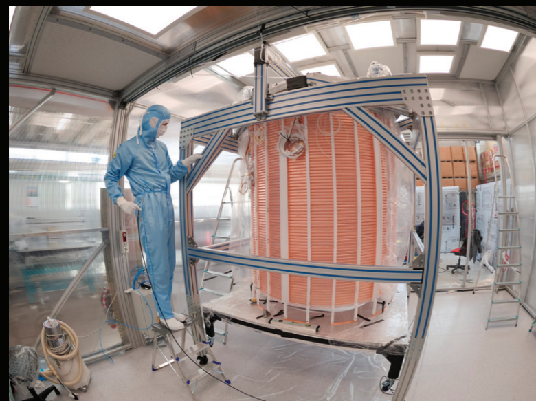
The XENONnT Detector during Assembly (Left) and Design (Right).
